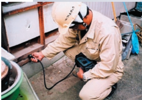
Compact and portable, “Wood Scan” identifies where hazardous CCA-containing lumber is used before a residential building is demolished.
