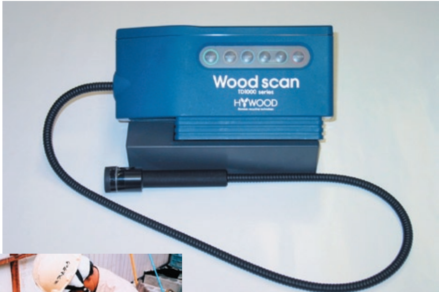
Compact and portable, “Wood Scan” identifies where hazardous CCA-containing lumber is used before a residential building is demolished.
